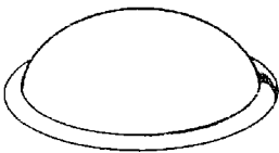
A DIAPHRAGM Made of a soft rubber dome with a rubber covered spring.
